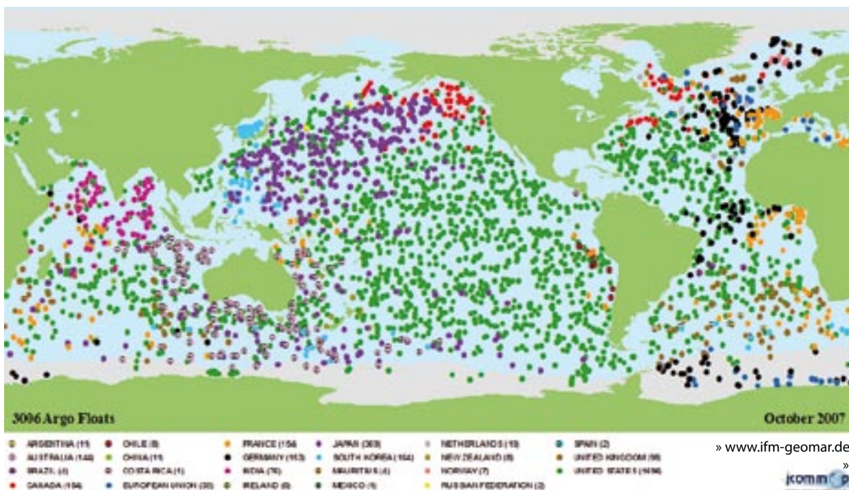
Figure 1: ARGO, a broad-scale global array with ~3,000 free-drifting profiling floats that measure the temperature of the oceans, providing data for weather and climate prognoses and for marine sciences.
